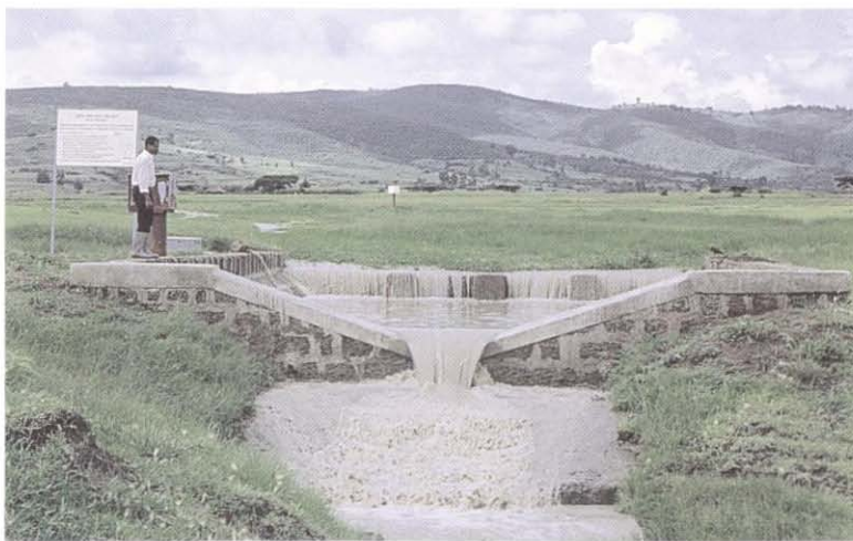
A V-notch device measures runoff at Ginchi.
