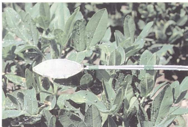
A leaf-shaped circuit board detects moisture.
