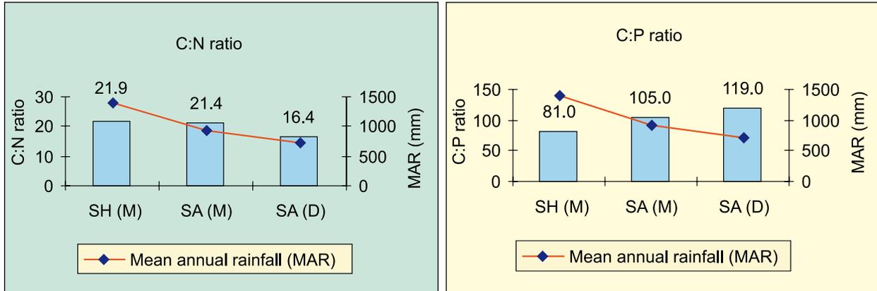
Figures 4.3 to 4.4 Variation in C:N and C:P ratios of red soils under different bioclimatic zones.
