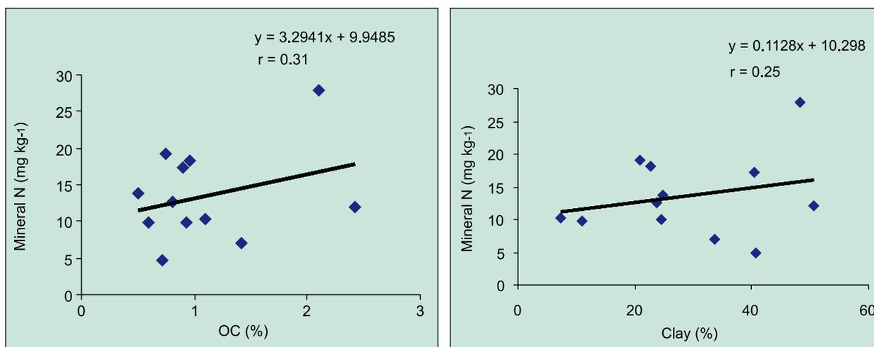
Figures 3.2.5 to 3.2.8. Relationship of various soil parameters with mineral N in red soils at 0–30 cm depth.
