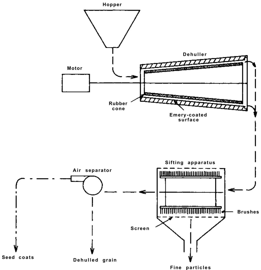
Figure 2. Schematic diagram of the FAO Eurafric dehuller. (Adapted from Munier 1980.)
