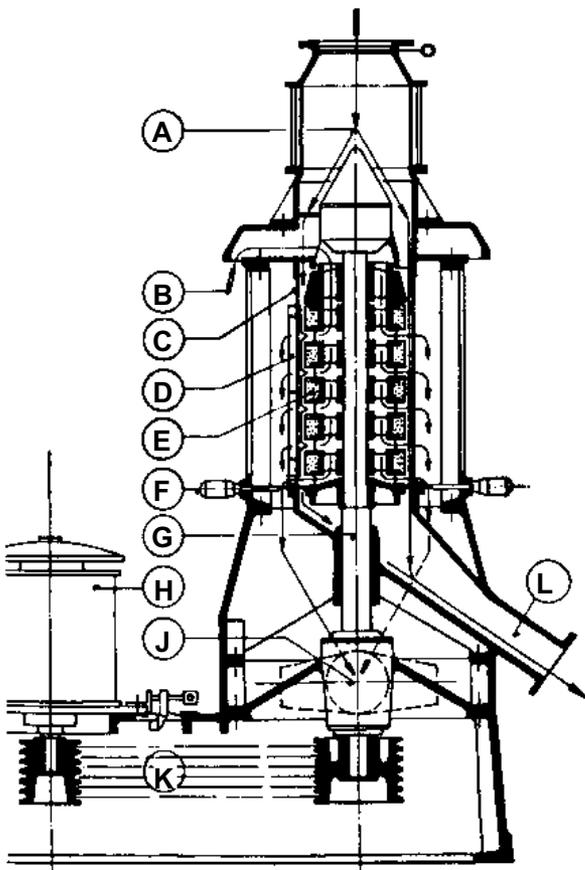
Figure 3 .Schematic diagram of the Decomatic dehuller. (Bernhard Keller AG literature.)
