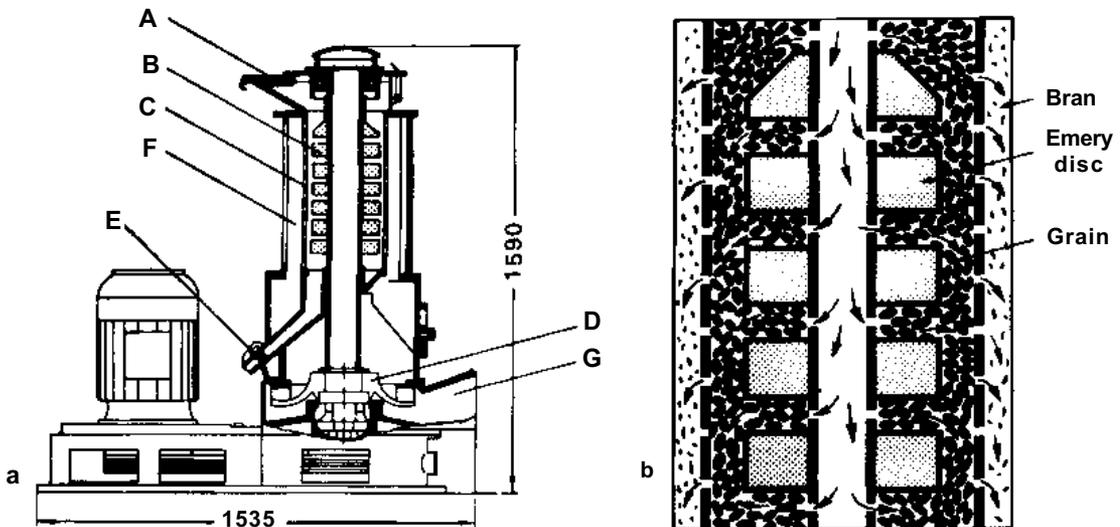
Figure 4. (a) Schematic diagram of the Vertical shelling type 270 machine (dimensions in mm); (b) magnified view of the working chamber illustrating the air and bran flow. (F.H. Schule GMBH literature.)
