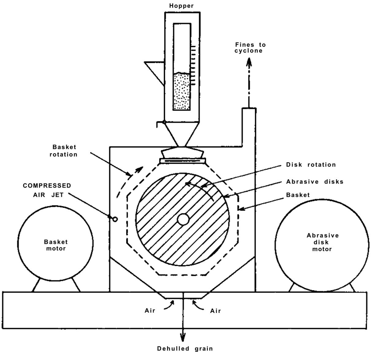
Figure 1. Schematic diagram of the Wondergrain Jaybee dehuller. (Adapted from Munier 1980.)
