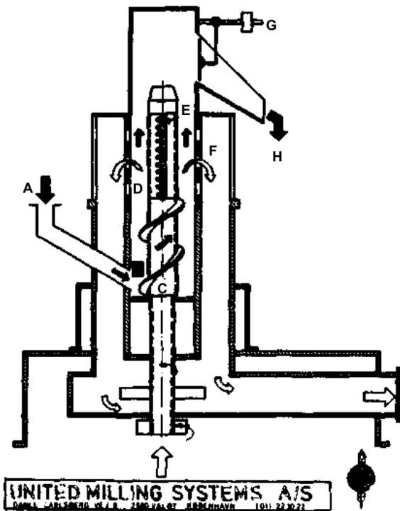
Figure 2. The United Milling Systems DVA sorghum dehuller (Munck et al. 1982).
