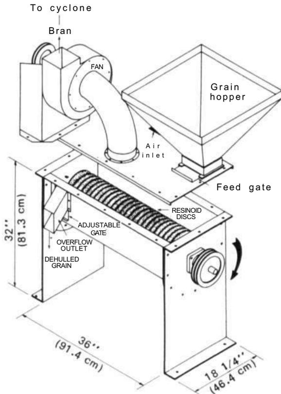
Figure 5. Schematic diagram of the PRL de-huller.
