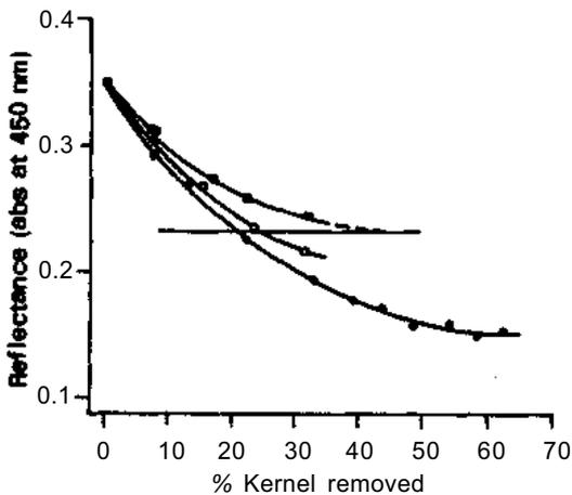
*Figure 9. Comparative rate of flour color improvement (reflectance measurement at 450 nm) as a function of progressive dehulling with laboratory (●), commercial abrasive-type (□), and attrition-type dehullers (■). Horizontal line represents a traditionally acceptable flour. (Reichert and Youngs 1976.)*
