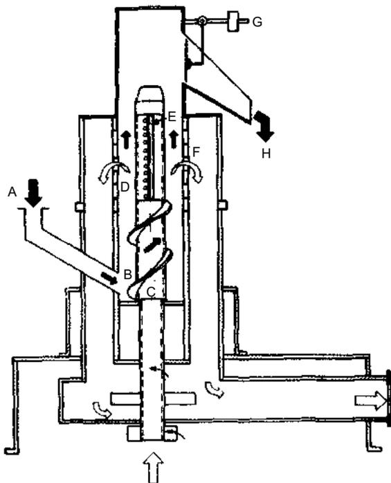
Figure 7. Schematic diagram of the UMS dehuller type DVA. (United Milling Systems literature.)
