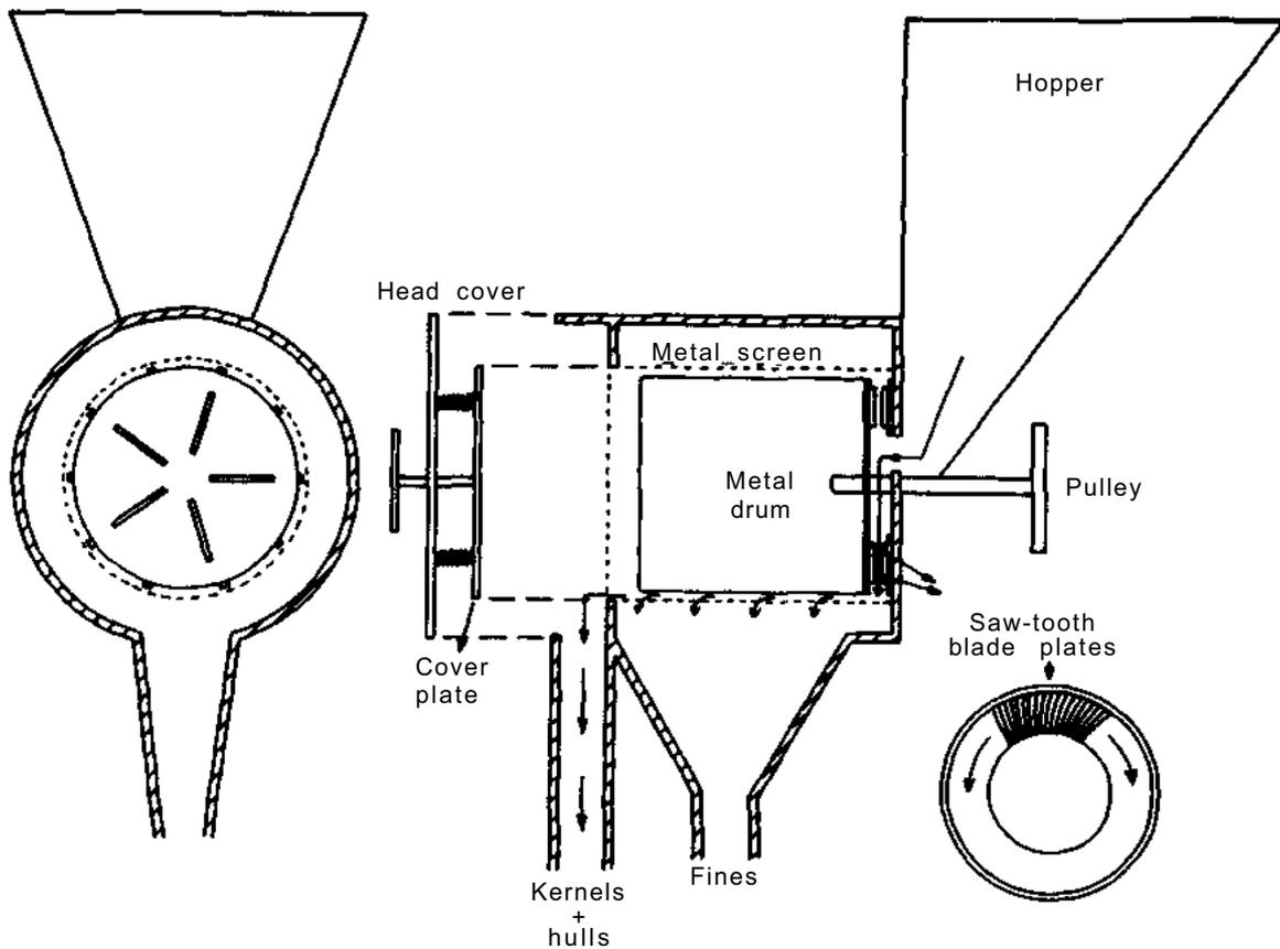
Figure 8. Schematic diagram of the front view (left) and side view (right) of the Palyi compact mill. (Reichert and Youngs 1976.)
