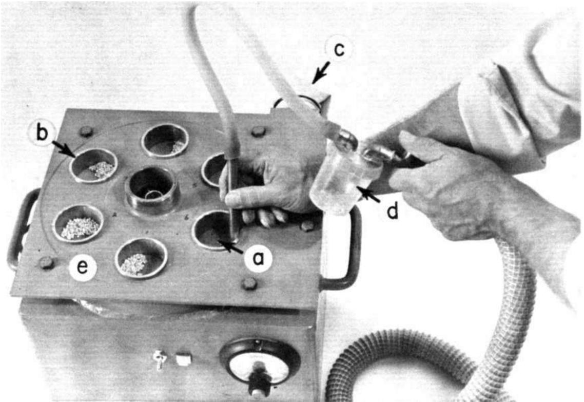
Figure 10. Photograph of the TADD used to predict dehulling quality. (Oomah et al. 1981.)
