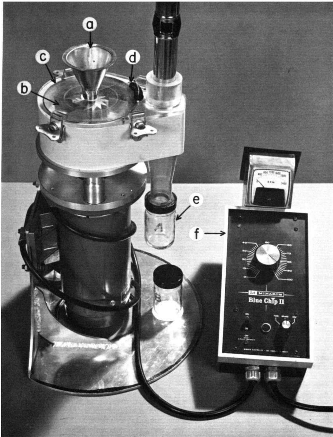
Figure 11. Photograph of the modified Udy cyclone mill used as a laboratory abrasive decorticating mill. (Shepherd 1979.)
