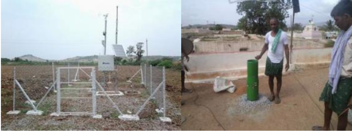
Figure 47. Automatic weather station installed in Chikkanthapur and one of the raingauges installed in Doddanthapur.
