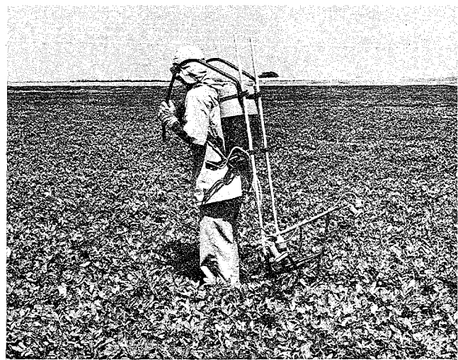
Figure 1. A twin spinning-disc, knapsack sprayer for groundnut and other low-growing crops.
