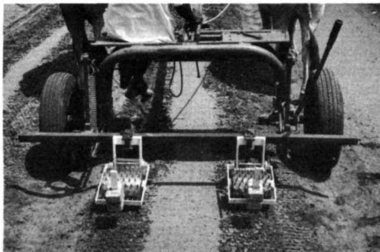
To break the crusts that reduce seedling emergence, ICRI-SAT engineers developed two models of a rolling crust breaker, one for hand operation and one for an animal-drawn wheeled tool carrier.
