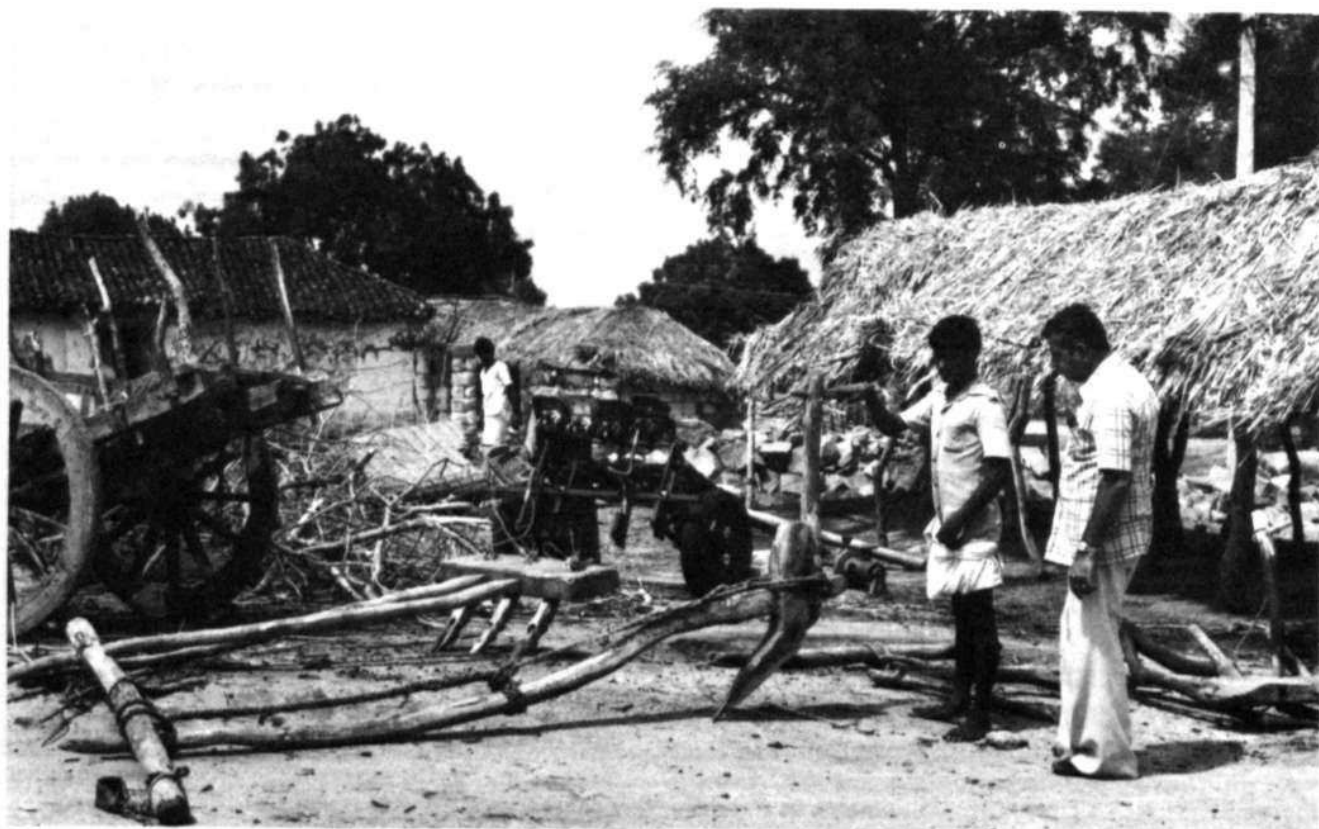
Traditional implements were used to perform a variety of functions in the Taddanpally experiment. Here seed is covered with a blade harrow after broadcasting. At bottom, an ICRISAT research technician discusses implements with a farmer. The weeled tool carrier is seen in the background.
