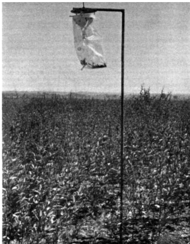
Pheromone traps modified with locally made materials from a design supplied by the Centre for Overseas Pest Research, London, effectively trap Heliothis armigera, the most damaging pest of pigeonpea. Much cheaper and easier to use than light traps, pheromone traps now are being used at 26 locations in India.
