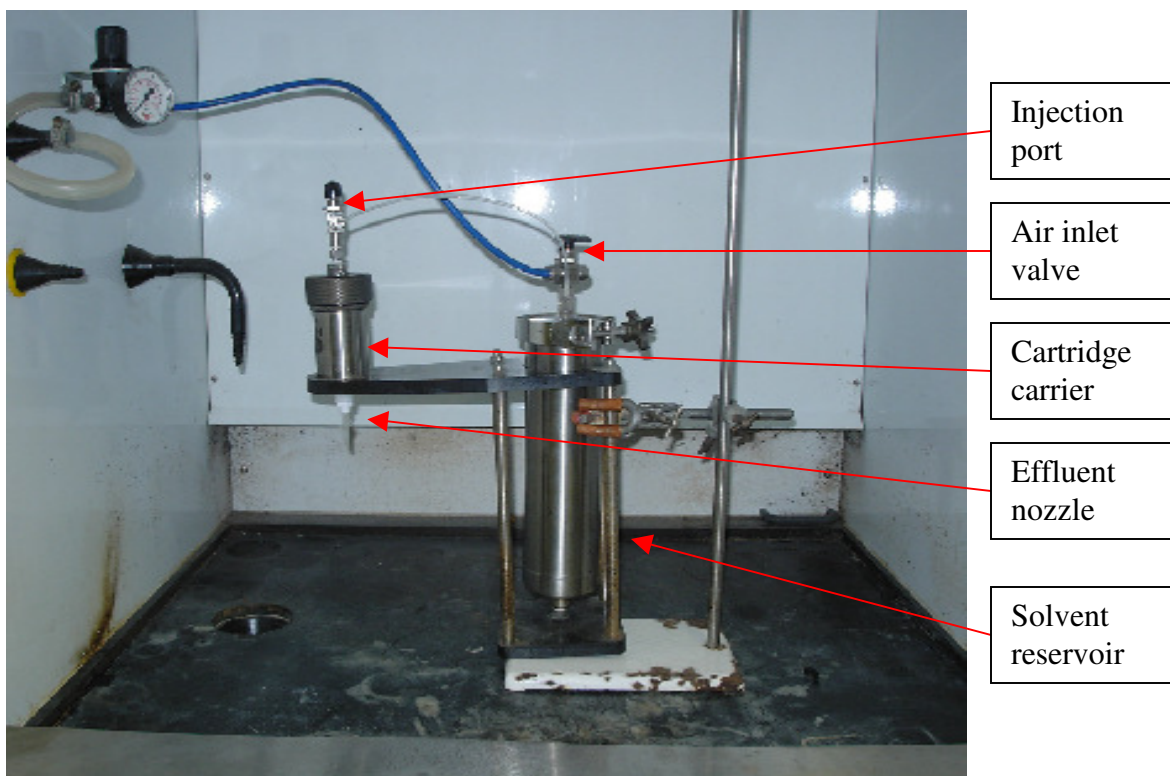
Fig. 5.1 The flash chromatography apparatus (Biotage UK Ltd., Hertford, UK) consisting of a solvent reservoir reservoir, a cylinder containing a disposable cartridge of pre-packed silica or C 18 resin and an injection port
