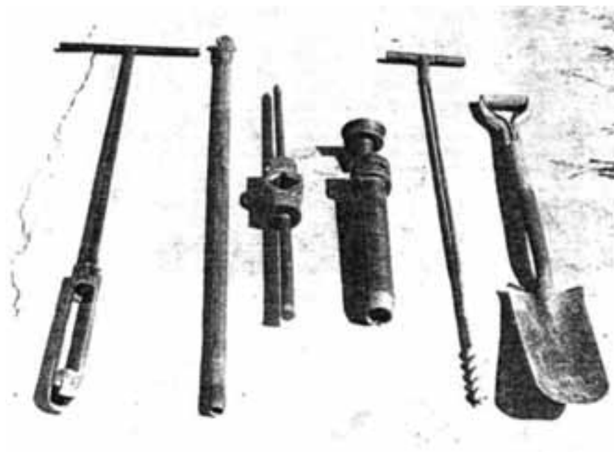
Figure 12. Soil sampling tools.
