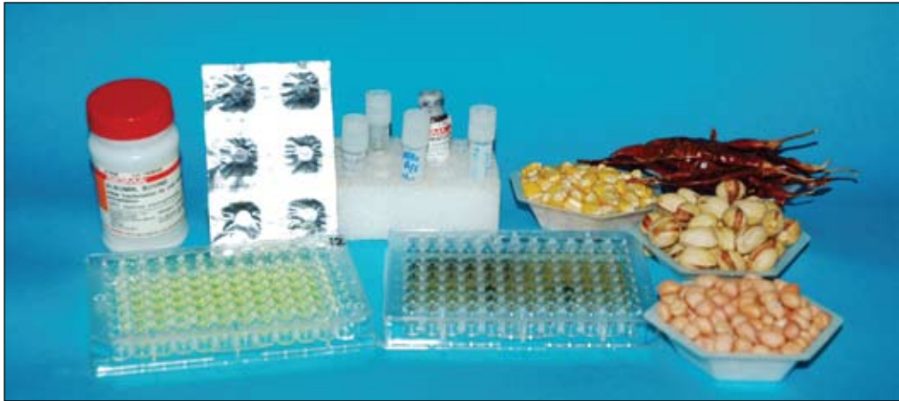
Figure 6. ELISA kit for mycotoxin detection in grain and feeds
