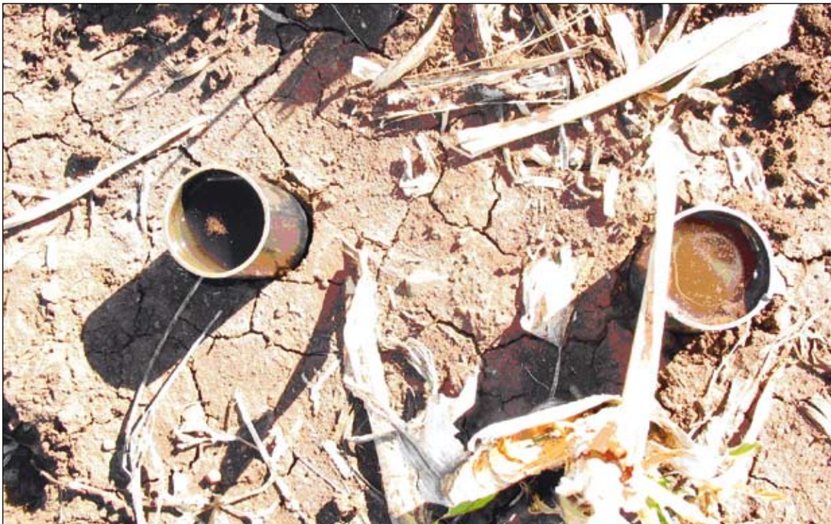
Plate 1. Infiltration measurements using steel cores (ponded method).
