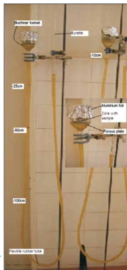
Plate 2. Hanging column method used to determine water retention.
