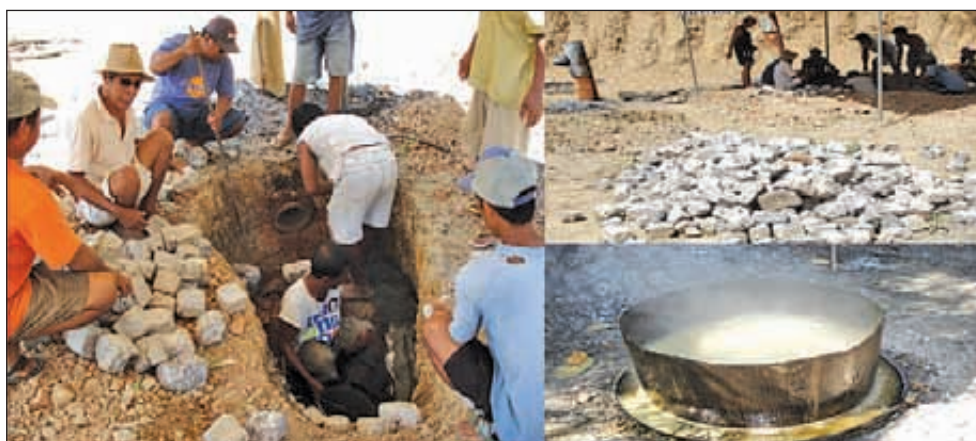
Figure 20. The construction and use of semi-permanent furnaces to pasteurize sweet sorghum juice.
