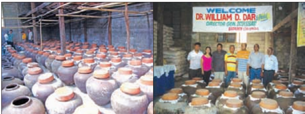
Figure 22. Earthen jars fermenting sweet sorghum juice into vinegar are housed in this warehouse-turned-fermentation center.
