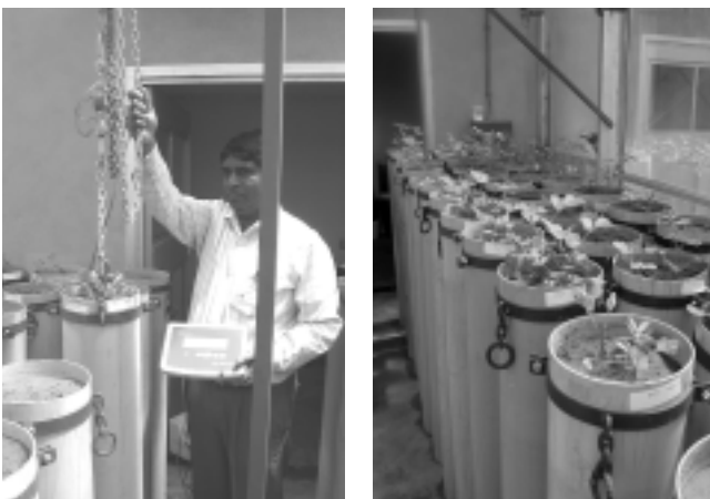
Fig. 6. Lysimetric system newly used at ICRISAT to evaluate plant water uptake in PVC tubes (1.2 m long, 20-cm diameter), filled with Alfisol at a bulk density of about 1.4. The length and diameter of the tubes are designed so that the soil volume available to each plant is equivalent to the soil volume available under field conditions at current sowing densities (for groundnut and chickpea). The system is used here for the evaluation of transgenics in P2 facilities.
