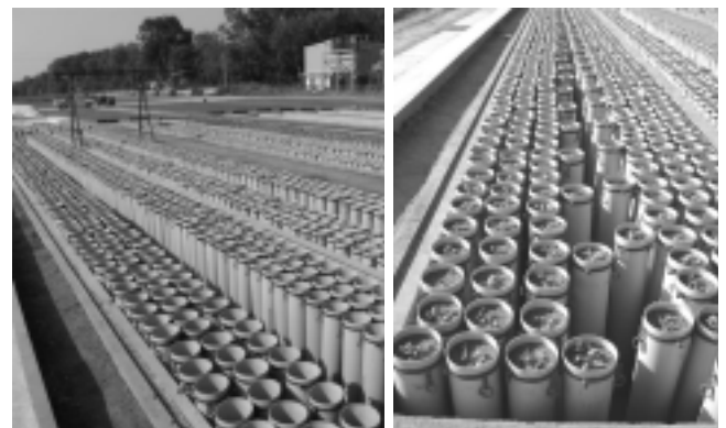
Fig. 7. Overall view of the lysimetric system developed at ICRISAT. The tubes are 1.2 m long with 20 cm diameter. They are filled with Alfisol at a set bulk density of 1.4. Each trench can accommodate approximately 700 cylinders. It takes about one day to 4 persons for weighing about 600 cylinders.
