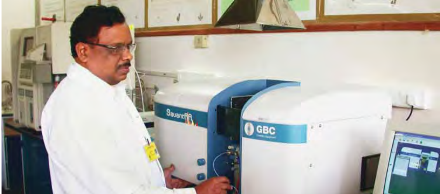
Estimation of macro and micro nutrients with an Atomic Absorption Spectrophotometer.
