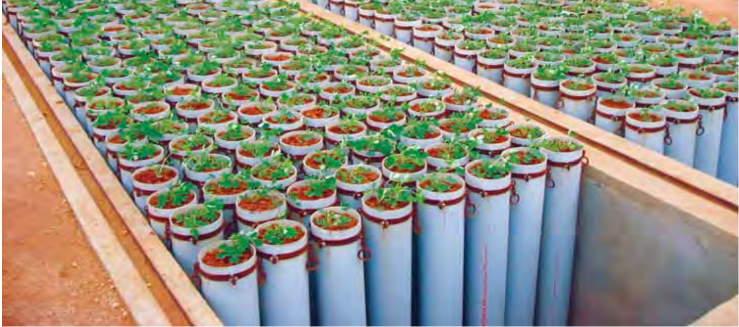
The large-scale lysimetric facility seen here with groundnut plants sown in cylinders.
