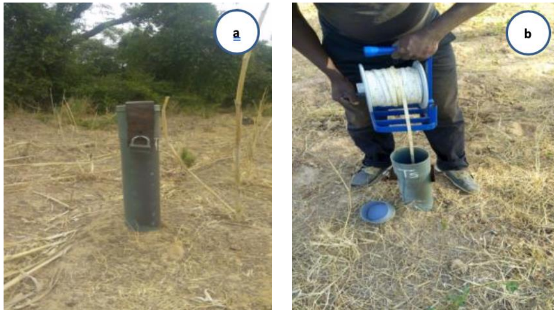
Photo 3: Measurement of water table dynamic, a) tube protected using a padlock, Noupinesso and Kani, 2018.) Photo credit: Kalifa Traore/IER.
