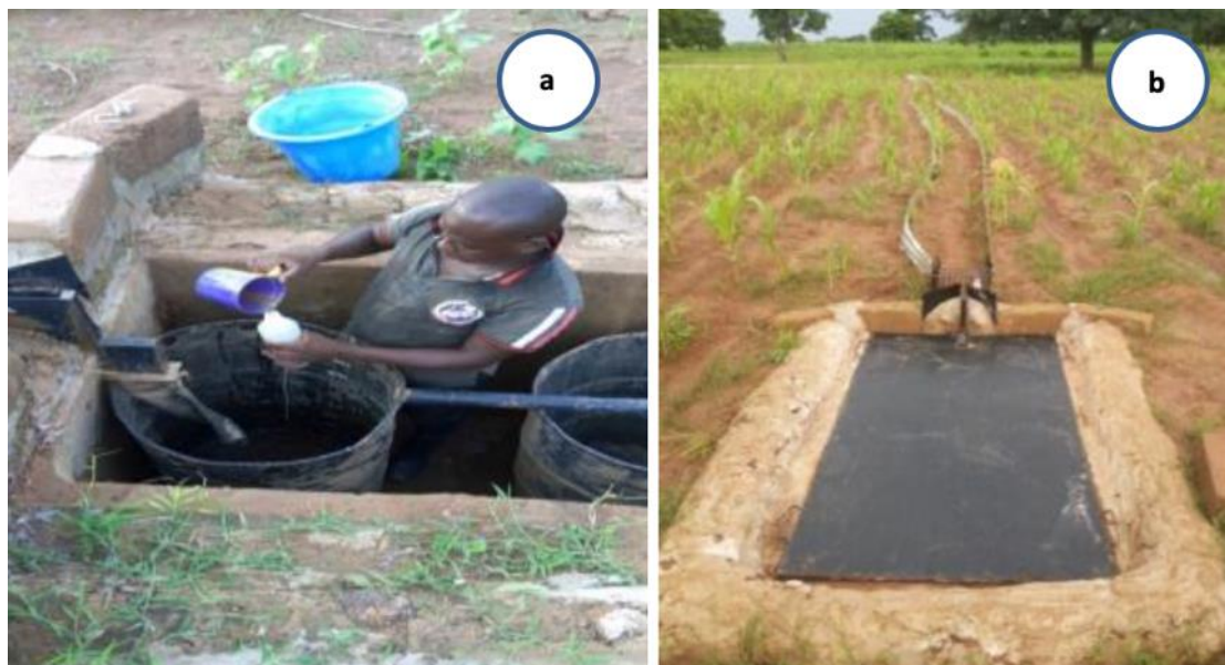
Photo 5: Device for measurement of runoff and erosion at Kani. Photo credit: Kalifa Traore/IER.
