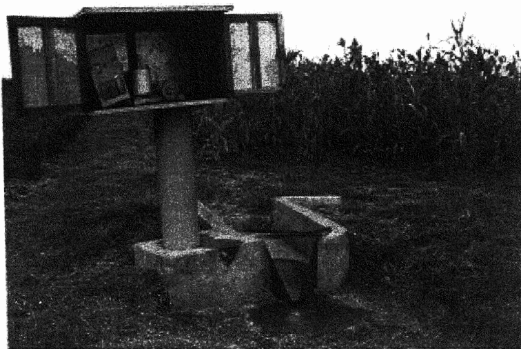
Plate 5 H-flume attached to a stilling well and connected to a drum type recorder for measuring runoff
