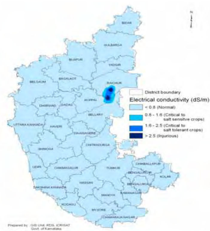
Figure 24. Soil Electrical Conductivity (EC) map of various soils in 30 districts of Karnataka, resulting from extrapolation of 92864 field samples analyses data during 2008-2011
