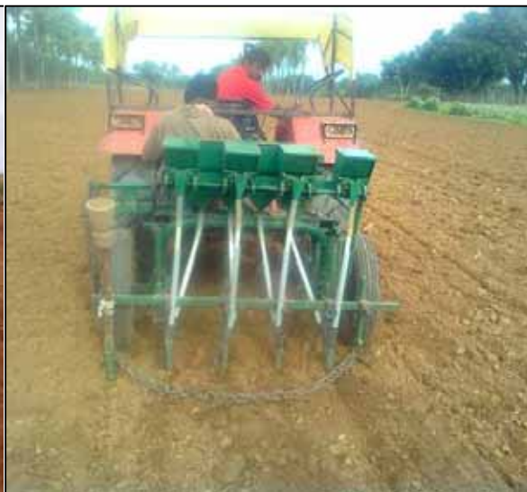
Figure 3b. Applying fertilizer and seed at a time with Tractor mounted Tropicultor in Kottur watershed, Dharwad
