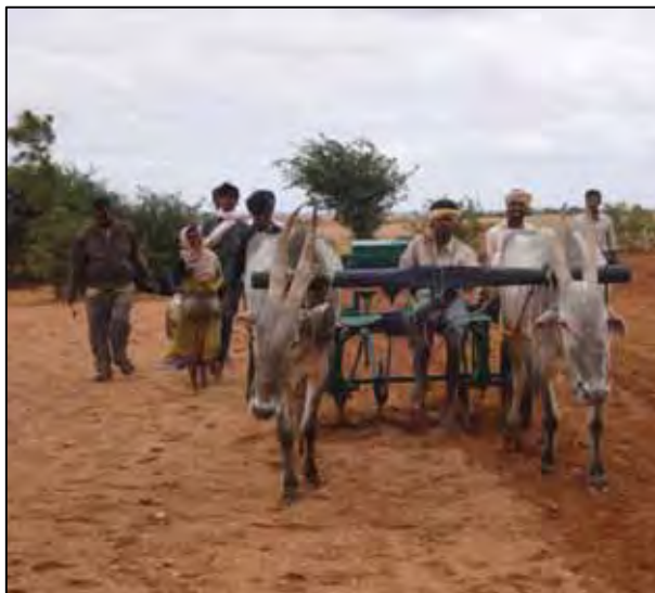
Figure 3a. Applying fertilizer and seed at a time with animal drawn Tropicultor
