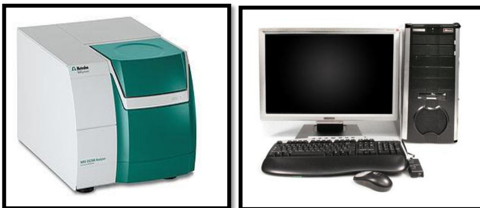
Plate 7. Near Infrared Reflectance Spectroscopy (NIRS) used for determination of oil and fatty acids in groundnut kernels
