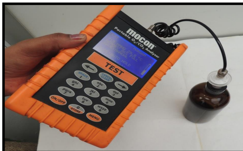
Plate 8B. Estimation of gas composition in septum bottles by using hand held Mocon head space analyser
