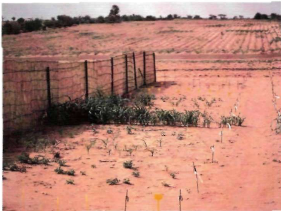
Heat trials at ISC using millet-stalk walls to vary soil temperature.
