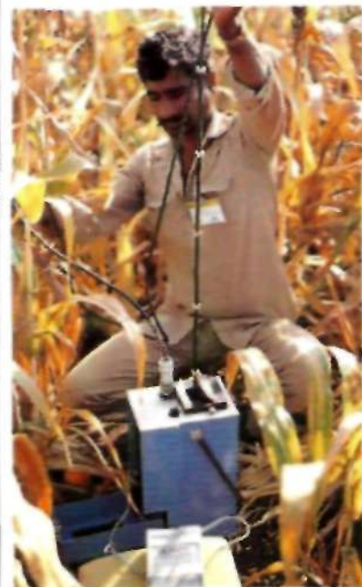
Field worker measures soil moisture using a neutron probe in sorghum grown in the post-rainy season.
