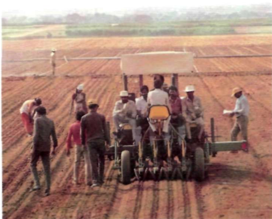
FDO personnel sowing groundnut on broadbeds with a vacuum planter.
