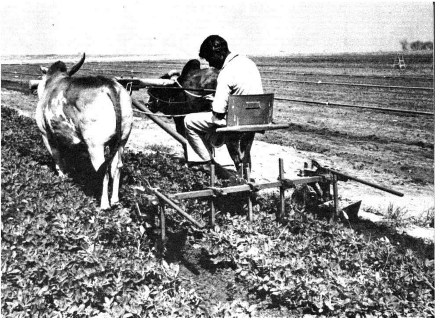
Figure 2. Interrow cultivation with duckfoot sweeps fitted on an Agribar II.
