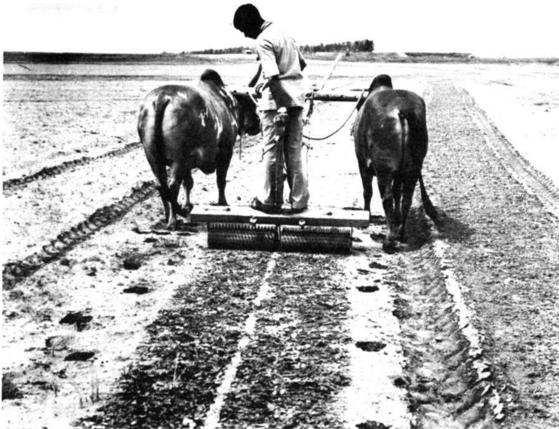
Figure 14. Inclined-roller crust breaker attached to a plank on an Alfisol, ICRISAT Center, 1986.
