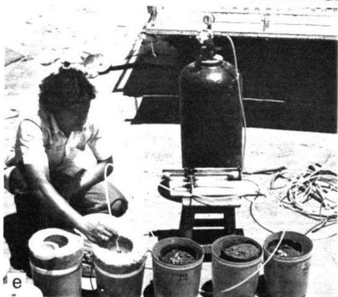
Figure 1. Steps in the soil-core assay technique for measuring nitrogenase activity of field-grown plants: (a) cutting plant at ground level and scraping of algal growth on soil surface; (b) driving metal core around plant roots; (c) lifting out soil-root core from the ground; (d) putting the soil core in plastic container; and (e) sealing container with PVC tape and injecting acetylene gas for incubation.
