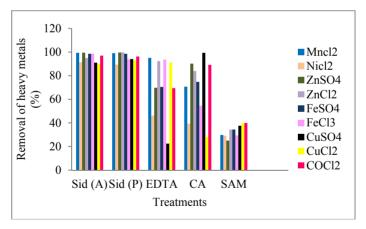
Fig. 7.3. Effect of sequential washing of heavy-metal-contaminated soil by washing agents
