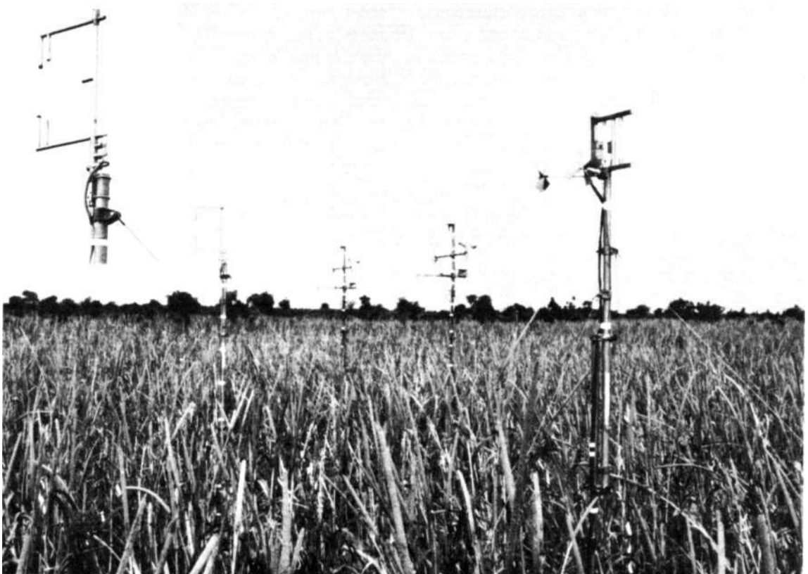
Figure 25. Measurement of evaporation from a pearl millet crop. Micrometeorological instrumentation from left to right, Hydra 2, two automatic weather stations, Hydra 1 (insert, enlarged Hydra 2). ISC, Niger, rainy season 1985.
