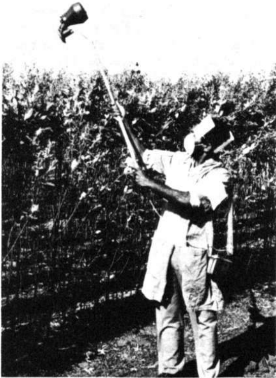
Figure 19. Technician testing the contamination hazard from droplet drift using a hand-held ULV sprayer on a pigeonpea crop. The spray contains a dye so that droplets drifting onto the body of the operator can be counted on the cards fixed to his clothing. ICRISAT Center, 1985.
