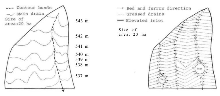
Figure 4. Topographic maps with contour intervals of 25-30 cm and a scale of 1:1000 to 1:2600 are most suitable for the design of land improvement plans.
