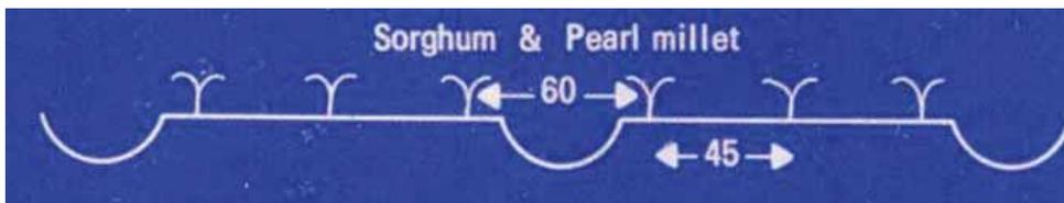
*Fig. 9. An illustration of the broad bed-and-furrow method.*
