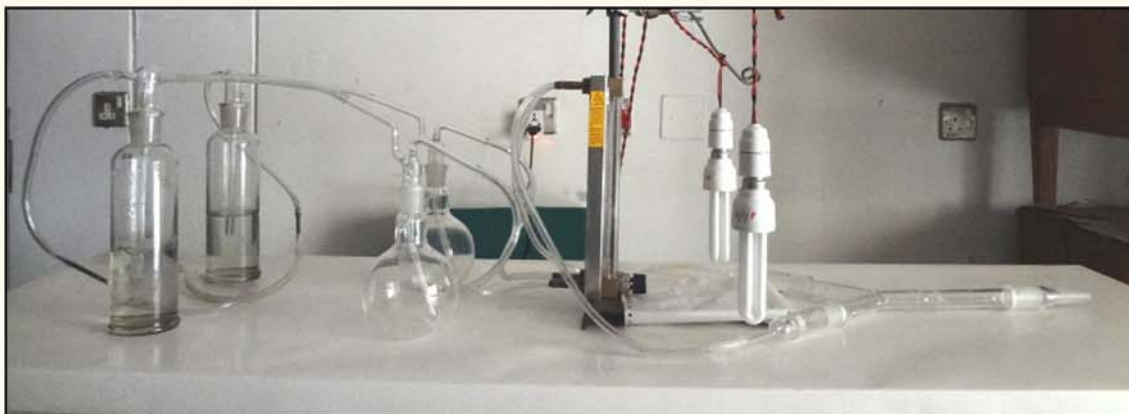
Olfactometer set-up used for attractant/repellent study of parasitoids
