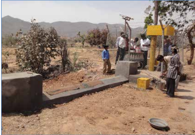
Figure 10. Digital runoff recorder, automatic sediment sampler installed at the Dob-Nevaj model watershed, Udaipur district
