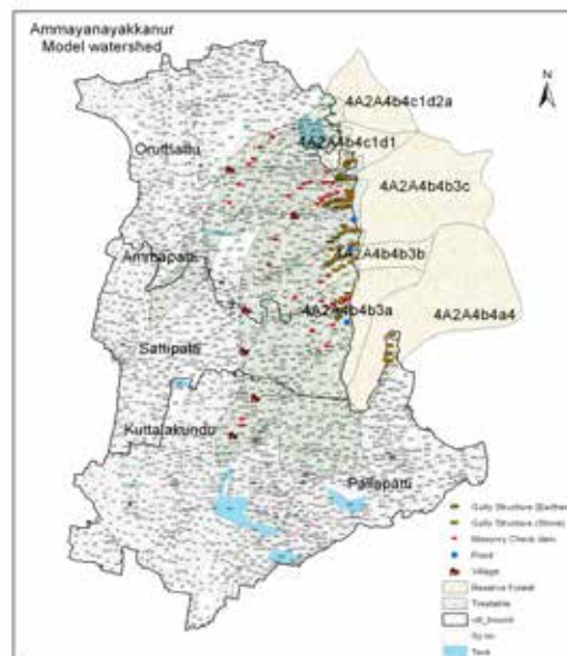
Figure 23. Proposed location of soil and water conservation structures
