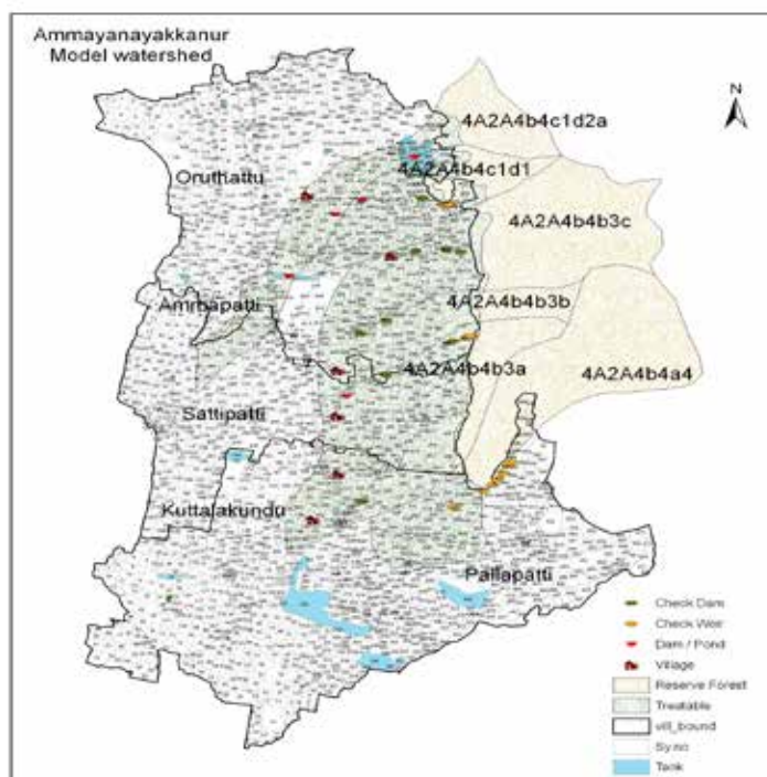
Figure 11. Location of existing soil conservation structures in Ammainaickanur model watershed
