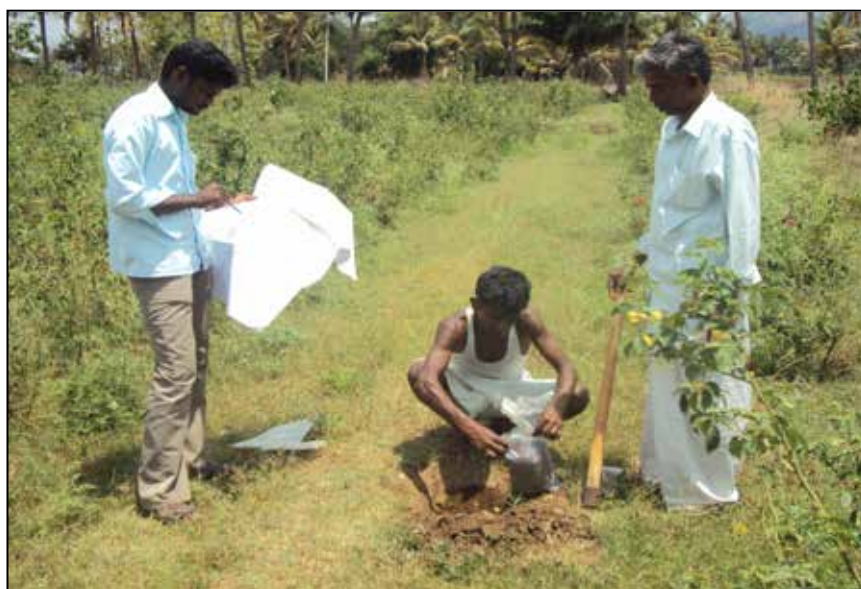
Figure 16. Collection of stratified soil samples in the Ammainaickanur watershed
