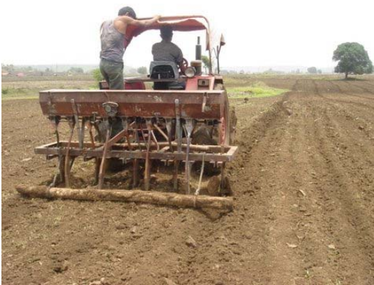
Tractor drawn BBF maker cum seed and fertilizer drill unit BBF formation, sowing, and good soybean crop in improved management system at Madhya Pradesh, 2011.
