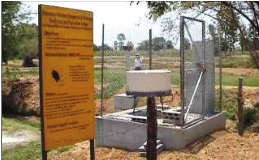
Figure 14. Hydrological monitoring station at Wang Chai watershed.
