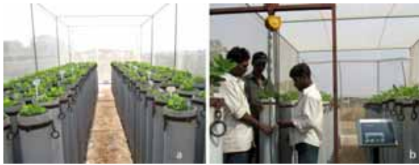
Figure 1. Experimental setup – confined outdoor trial using the lysimeters: (a) two sets of cylinders arranged according to RCBD design in a net enclosure; and (b) weighing balance and pulley.
