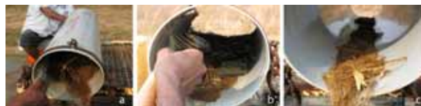
Figure 2. Complete root extraction from the lysimeters: (a) washing away soil from both ends; (b) most of the soil washed off; and (c) complete root extracted along the length of the cylinder.
