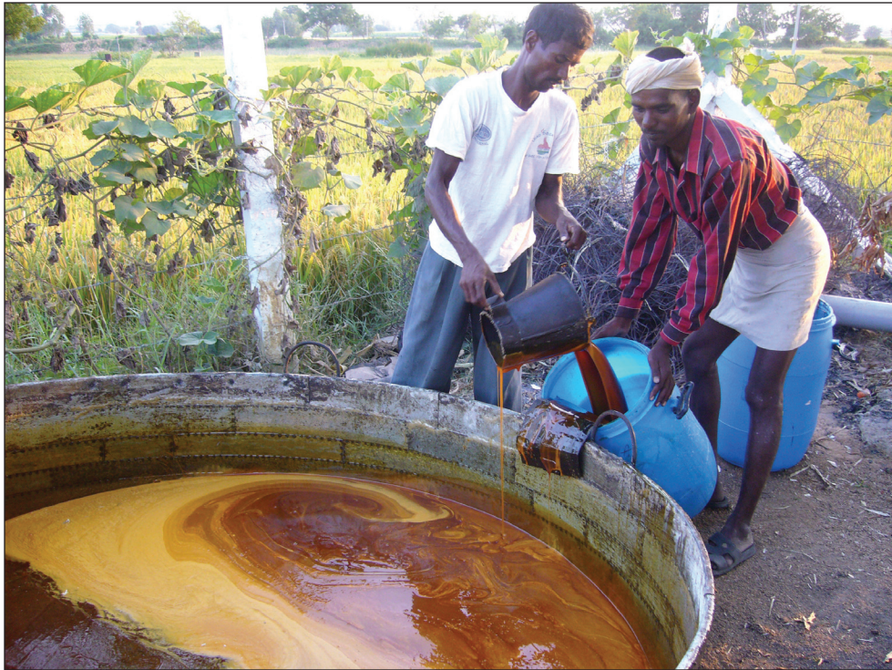
Figure 6. Syrup from pans are poured into wide-mouthed syrup storage cans.
