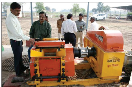
Sugarcane crusher with modified rollers.
