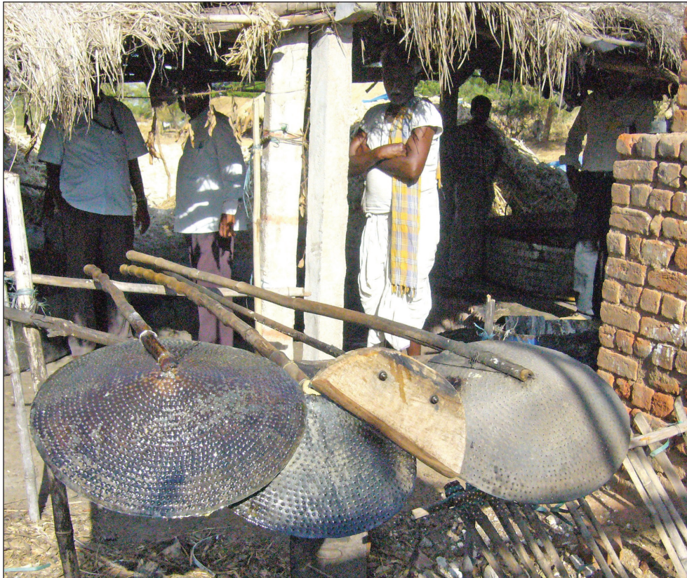
Figure 5. Juice boiling accessories, metal sieves and wooden dragger.
