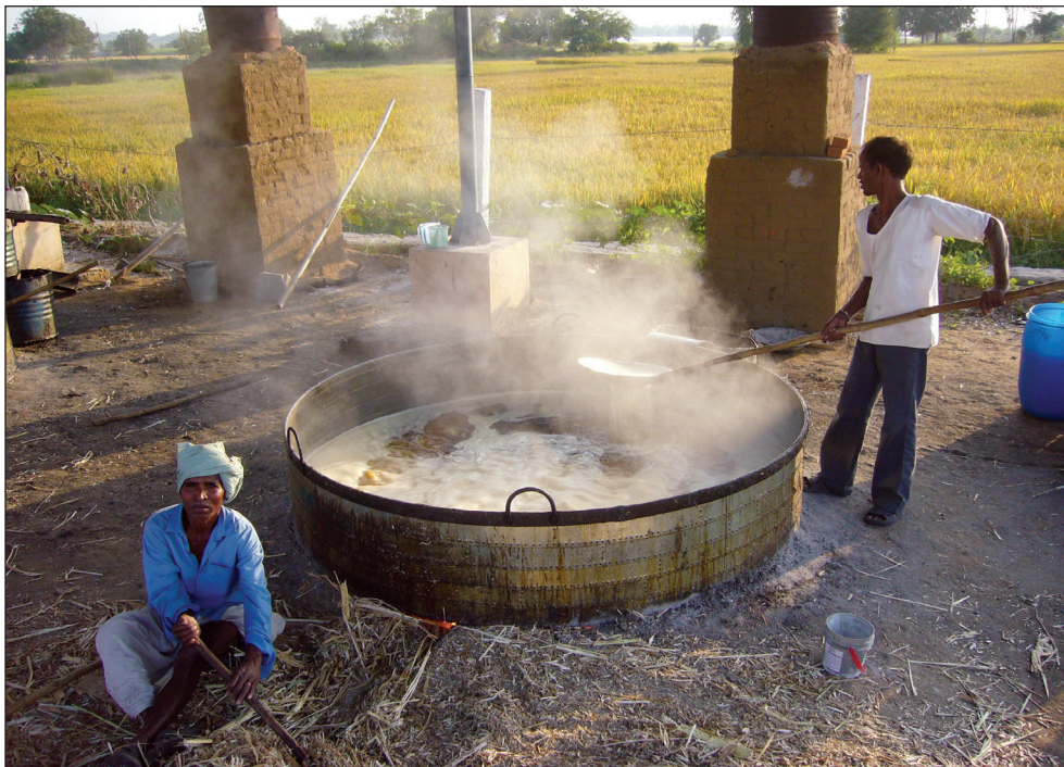
Figure 4. Boiling juice in the pan and feeding bagasse into the chulha.
