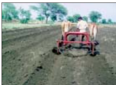
Figure 6. Broad-bed and furrow landform constructed with the tropiculator.
