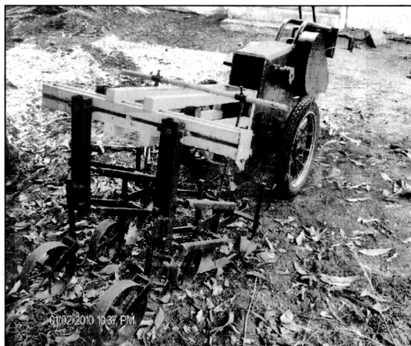
Fig. 3: Sweep blade type power tiller
