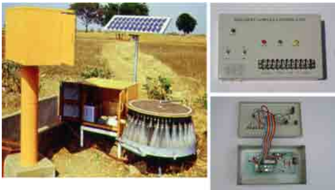
Fig 13. Hydrological monitoring station with runoff recorder and sediment sampler and control unit.
