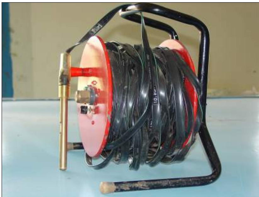
Fig14. Well water measuring device.
