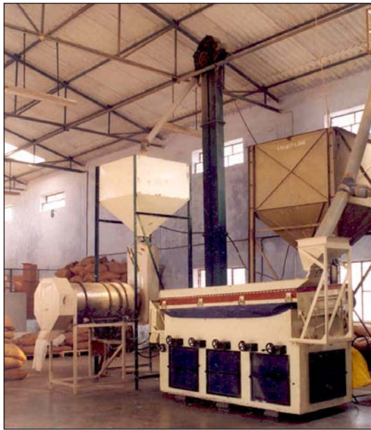
Fig. 31. A view of seed pre-cleaner cum grader and specific gravity and indented cylinder separators.
