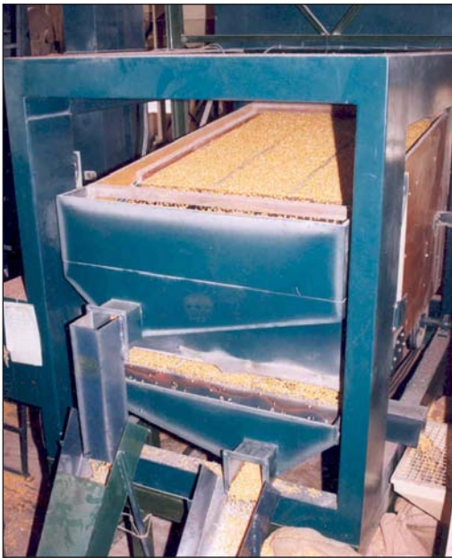
Fig. 31. A view of seed pre-cleaner cum grader and specific gravity and indented cylinder separators.
