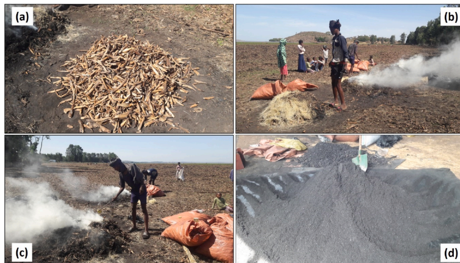
Fig. 1. Water hyacinth biochar preparation (a) water hyacinth biomass collection, (b) covering up the weed biomass with teff straw and soil, (c) carbonization process of the biomass, and (d) sieved biochar prepared for field application.
