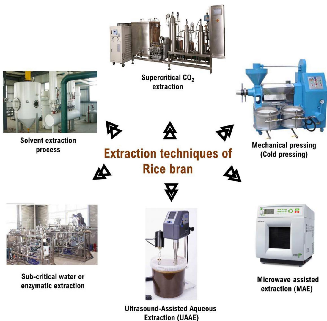
Figure 3. Different Methods and Instrumentation Technologies Utilized for Rice Bran Extraction. Solvent extraction (methanol, ethanol, hexane) utilizes a Soxhlet extractor or similar apparatus to dissolve oils and bioactive compounds. Mechanical pressing (cold pressing) uses a cold press machine to physically extract oil. Microwave-assisted extraction uses a microwave reactor to enhance extraction efficiency. Ultrasound-assisted aqueous extraction uses an ultrasonic bath or probe to disrupt cell walls and facilitate the release of bioactive compounds. Sub-critical water or enzymatic extraction involves a high-pressure reactor for sub-critical water extraction or a bioreactor for enzymatic hydrolysis. Supercritical fluid extraction utilizes a supercritical CO 2 extractor to obtain pure extracts
