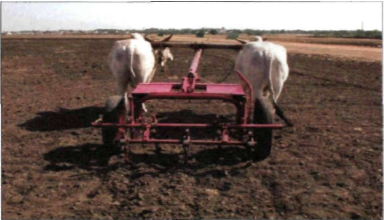
Figure 31. The animal-drawn tool carrier (tropicultor) developed by ICRISAT for Indian vertisols, facilitates speedier and precise tilling and planting.
