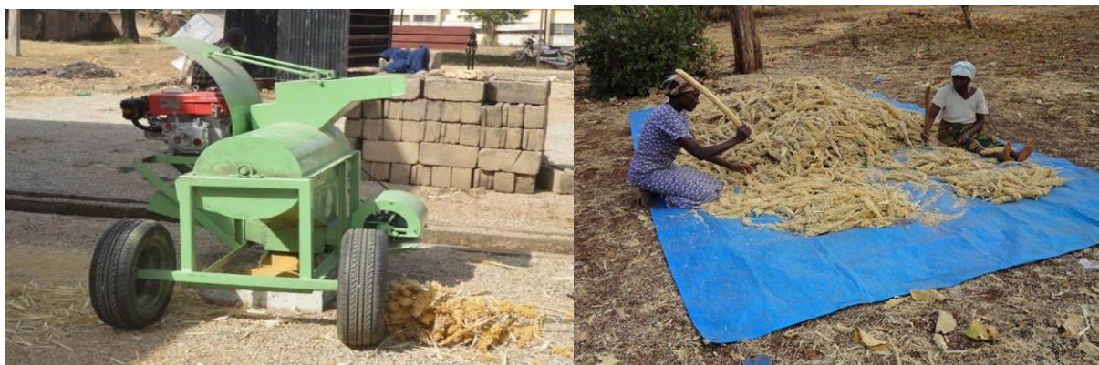
Plate 6: (L) A motorized multi-crop thresher and (R) manual threshing of sorghum.
