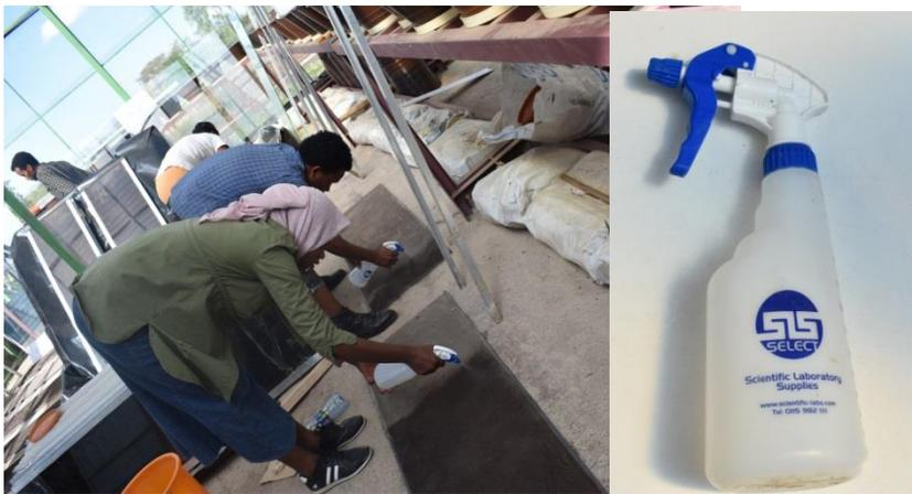
**Figure 2.** Moistening the soil using spray funnel
