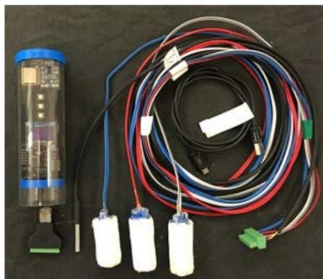
**Figure 6.** Chameleon™ soil moisture sensors and reader (Photo: VIA Farm website)
