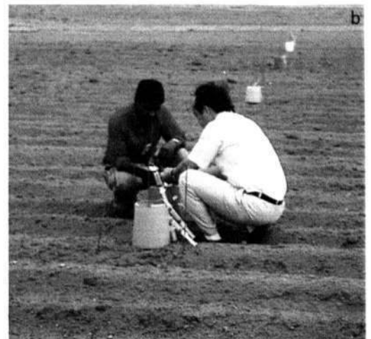
Figure 3. Development of the 'porous cup' method (a) enabled non-destructive detailed point sampling (b) of soil solutions
