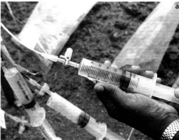
Figure 3. Development of the 'porous cup' method (a) enabled non-destructive detailed point sampling (b) of soil solutions
