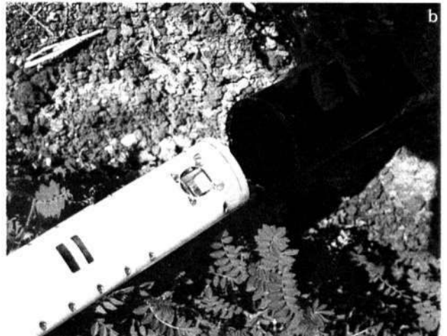
Figure 2. By Phase II the minirhizotron (a) could send a tiny video camera (b) into the soil to view roots in situ
