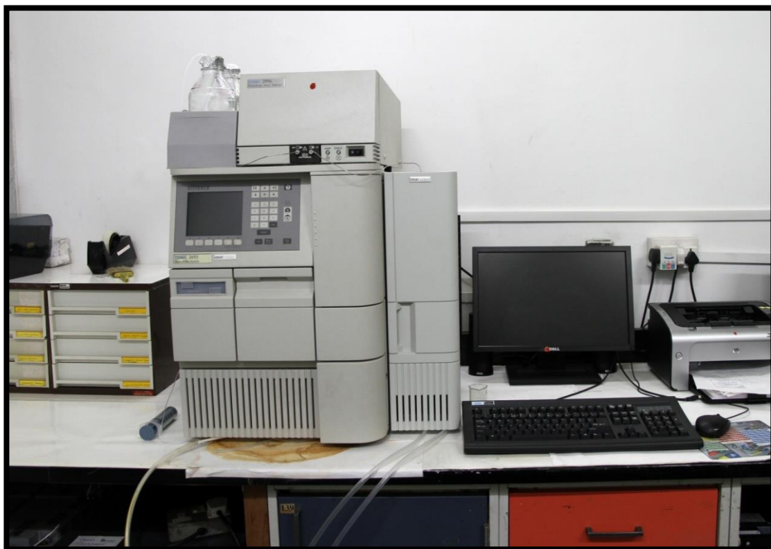
Plate 7. HPLC used for estimation of leaf organic acids and flavonoids
