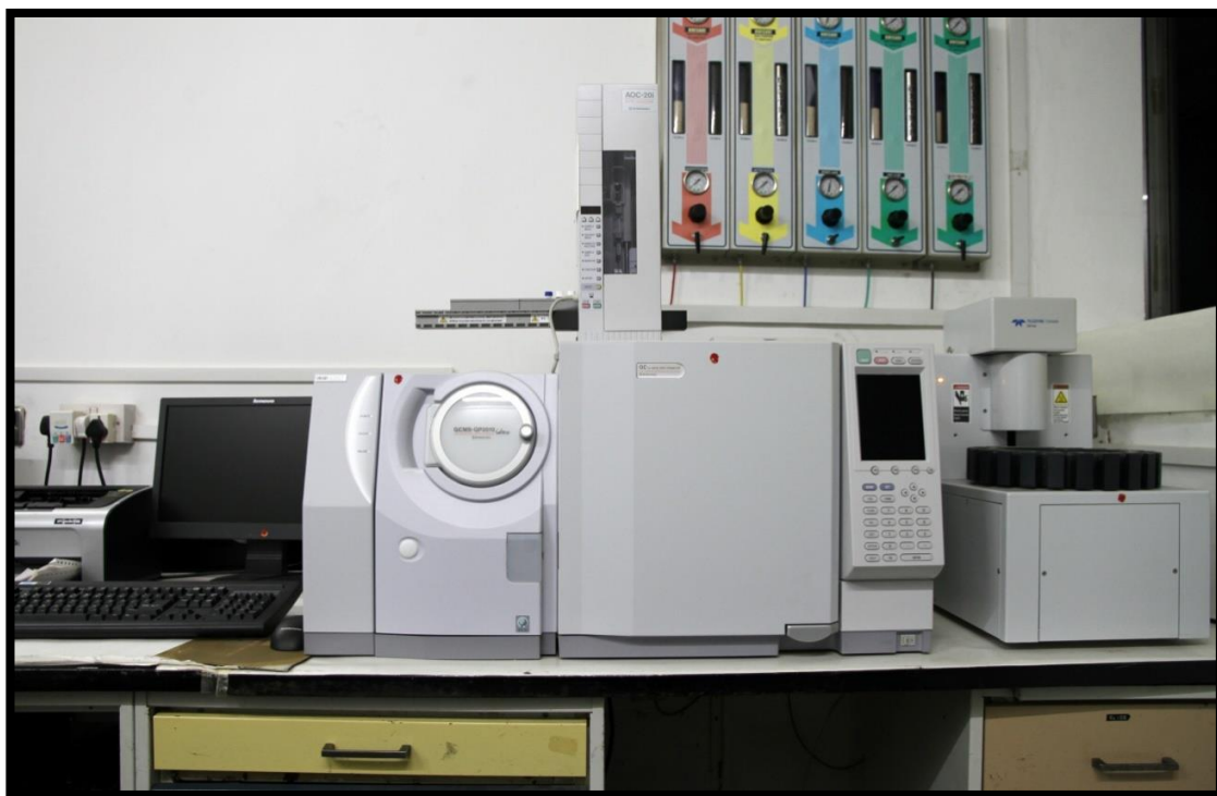
Plate 8. GC-MS used for estimation of leaf surface chemicals through hexane and methanol extracts
