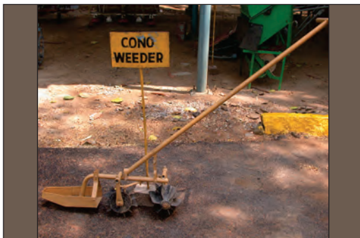
Plate 23. Cono weeder for different soils
