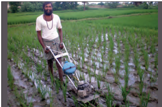
Plate 26. Motorised weeder operated by farmer (Mr. Gopala Swamy)
