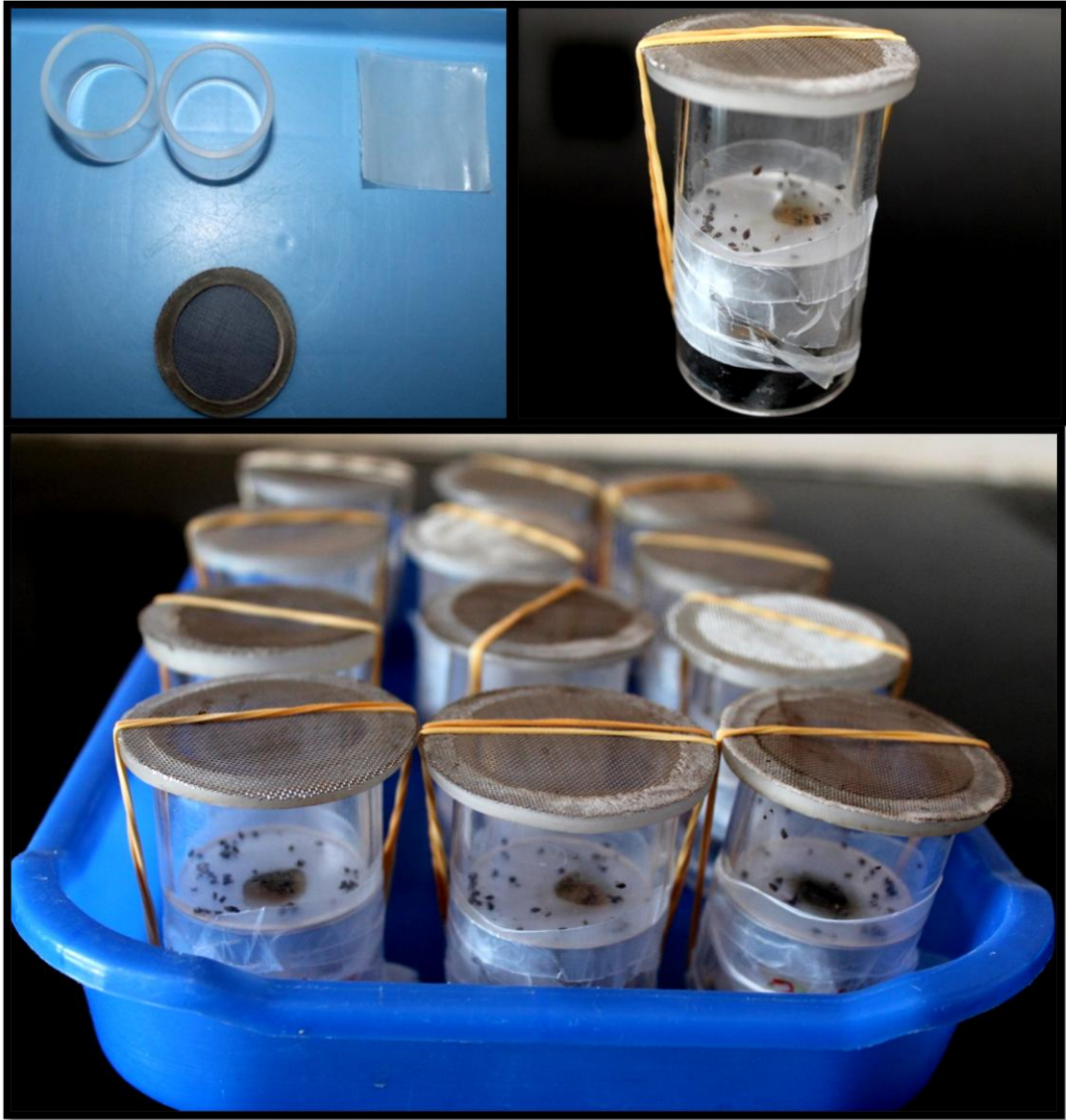
Plate 10: Aphid feeding apparatus
